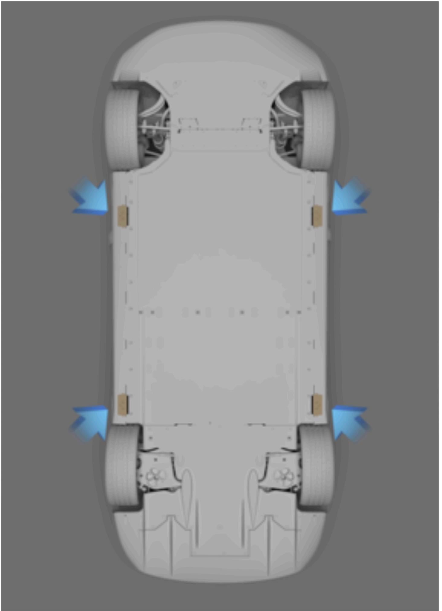
Ensure that any non-Lucid repair facility servicing your vehicle is aware of these lifting points when raising your vehicle on a lift.
